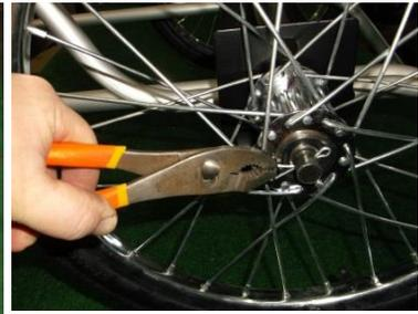
Install the axle through the cross brace by first removing one of the vinyl caps, then sliding it through a wheel and then the appropriate hole for your wheel size (see picture above). The cotter pins needs to be opened and bent in order to stay secured.
