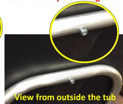
8.1: Make sure that your tub is centered within your frame and drill a hole above the two tub kick-outs (back and front of the cart) going through the pre-drilled holes in the aluminum frame. You would need a  $\frac{1}{4}$ " size drill bit and a powered drill.
