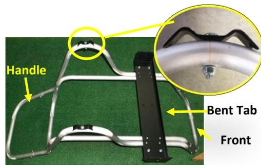
The holes will not align properly if the cross brace faces backward. The cross brace bent tab has to be installed to be close to the front of the frame and the farthest away from the Handle.
